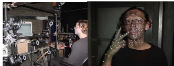
Figure 4: Motion capture using a VICON® system with 12 cameras, 50 beads glued on the hand and 63 on the face.
