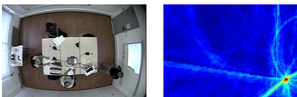
Figure 1: On the left, zenithal camera snapshot. On the right, example of the Sound Map obtained with the SRP-PHAT process.
