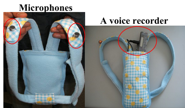
Figure 2. A wearable speech recording device.
